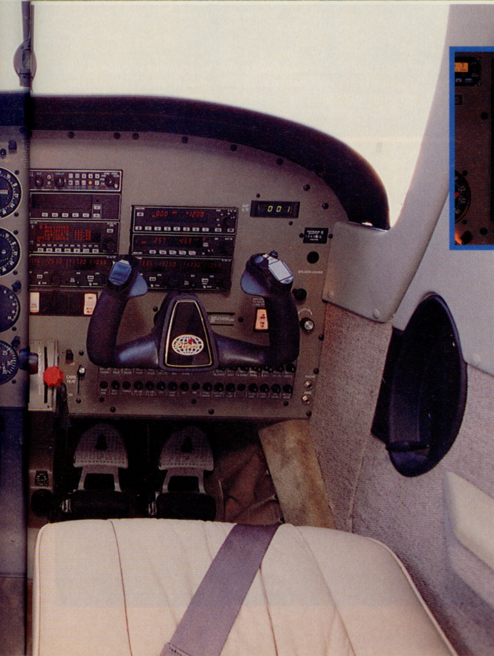
The current Bendix/King Silver Crown Plus avionics (left) will be replaced by a stack of radios from Garmin and topped off with an S-Tec autopilot (above).
