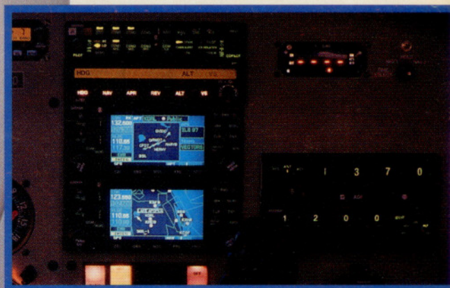
The current Bendix/King Silver Crown Plus avionics (left) will be replaced by a stack of radios from Garmin and topped off with an S-Tec autopilot (above).
